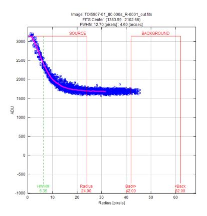
After, we used multi-aperture photometry to generate our measurement table used to generate the lightcurve. Then, we used the star's stellar surface gravity, effective temperature, and metallicity to determine the Linear LD u1 and Quad LD u2 values. Using the data value we created the lightcurve.
